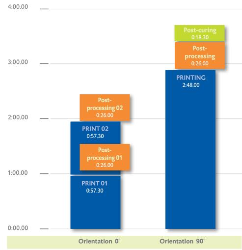
Time required in hours for the 3D printing of 6 splints in the validated DentaMile workflow in 0° (left) and 90° orientation (right). When printing 6 splints in a flat orientation, you can save more than one hour compared to printing in a vertical orientation.
